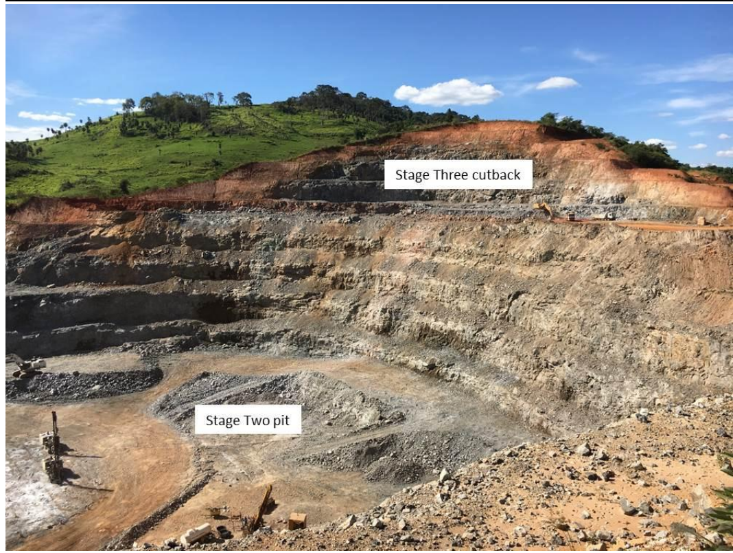
Figure 2: Active mining in Stage Two & cutting back on Stage Three at Antas
