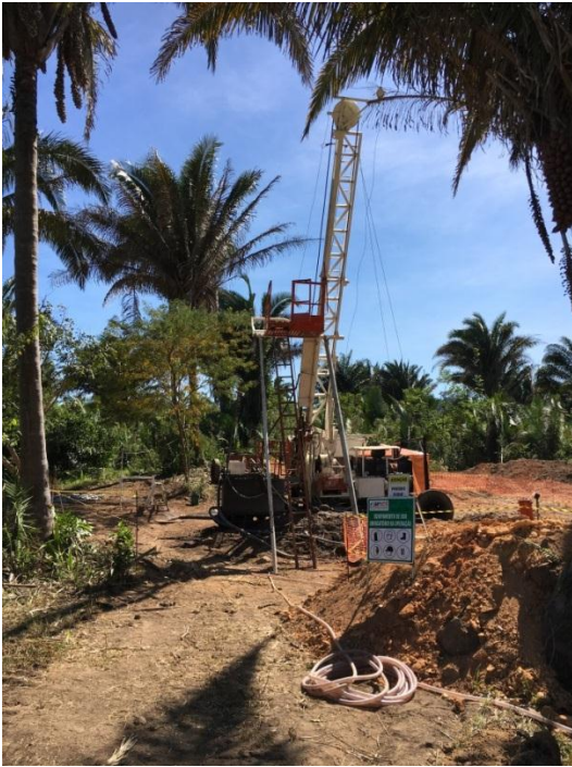
Figure 12: Diamond drilling at Petra Branca
