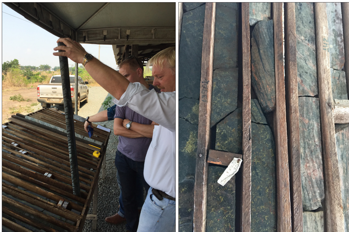
PB East drill core. Competent granite host and sharp contact.
